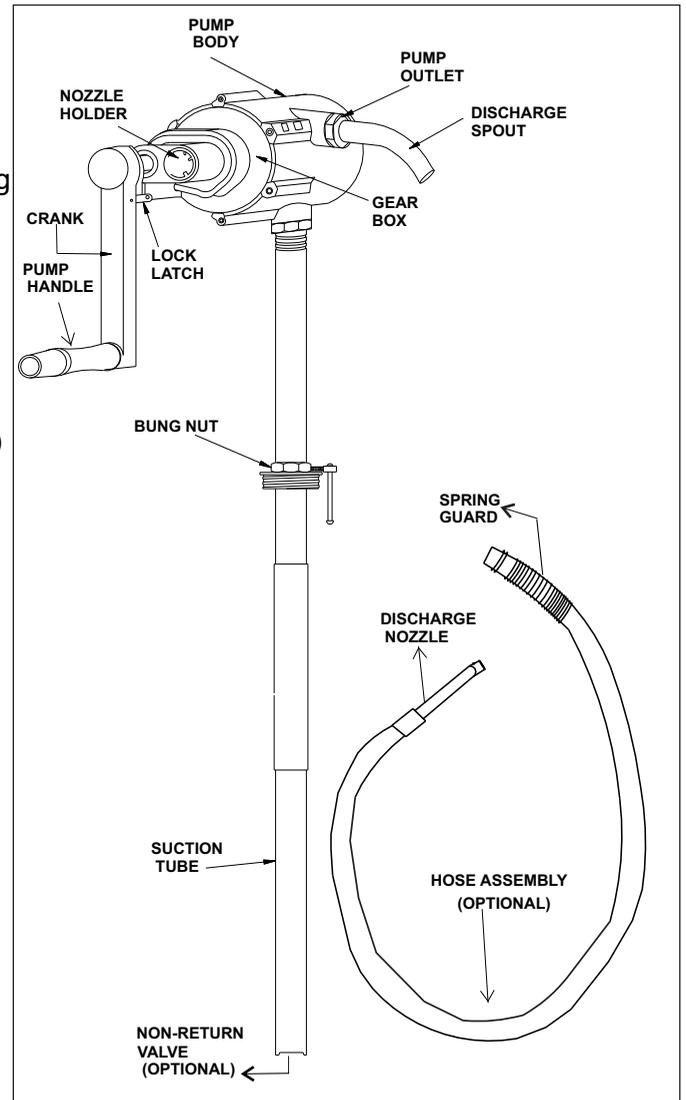
5. Tighten the suction tube onto the pump inlet. It is good practice to use a sealant such as Teflon in connecting the suction tube to the pump inlet
